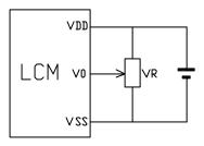
$V_{DD}$ -V<sub>0</sub>: LCD Driving voltage VR: 10k-20k
